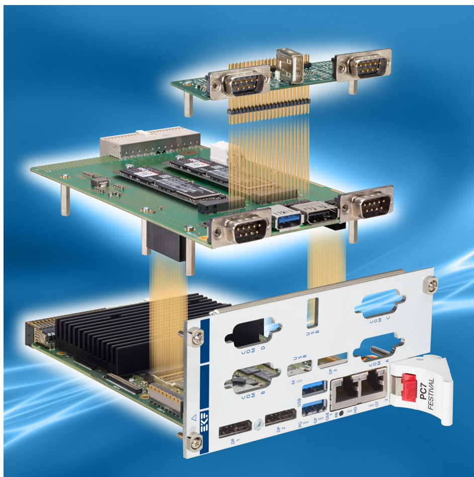
12HP Assembly w. PCZ-NVM & C32-FIO
